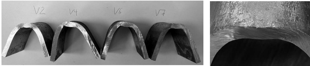
Fig. 16 Bottom-side specimens with no fracture after testing. The plastic flow of material around the HAZ is observed.
