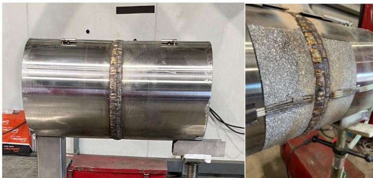
Fig. 7 Austenitic steel pipe mock-up with thermocouples instrumentation and speckles for stereo correlation analysis
