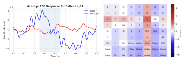
Figure 2: (Left) Average electroencephalography (EEG) signals from participant L_03 following target and non-target stimuli. A characteristic positive peak at approximately 270 ms is observed for target stimuli relative to non-target stimuli. (Right) Heatmap of character scores following cumulative P300 classifier score updates; character "V" receives the highest score and is selected as the user's intended character [2].
