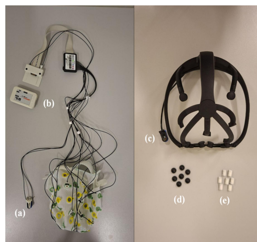
Figure 1: Image of EasyCap (on the left), with the earclip (a) and the LiveAmp amplifier (b) and X.on (on the right), with the earclip (c), sponges (e) and their holders (d).
