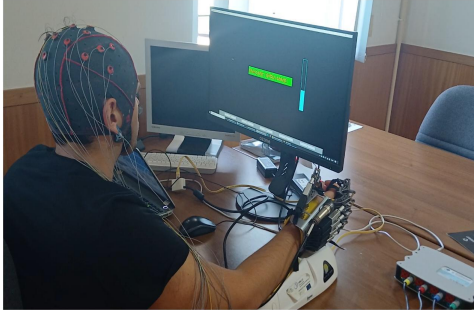
Figure 2: Experimental setup including the EEG acquisition system, the visual interface, and the robotic hand (Hand Of Hope).
