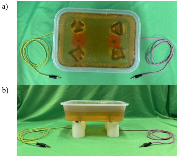
Figure 2: a) Top and b) side view of gelatin-based skin phantom with embedded electrodes
