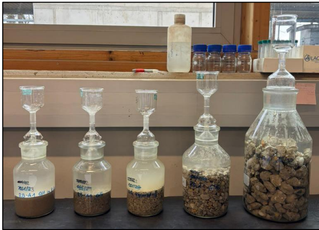
Figure 2 (Left) Water absorption capacity and OD density measurement using pycnometer according to ÖN EN 1097-6 and (Right) water absorption capacity over time of different aggregate sizes
