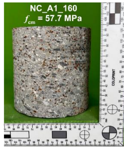
Figure 7: NC_A1_160 drilled core from boxes sprayed with 7% of accelerator.
