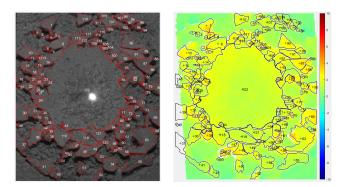
Fig. 9. Depth map at the end of cleaning, in mm (right). From camera view, gravity goes up. Numbered patches (red outlines).
