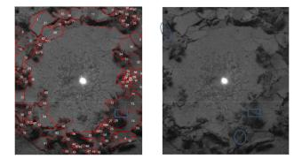
Fig. 10. Stereo images of back (left) and front (right) camera at end of detatchment process. From camera view, gravity goes up. All annotated patches are numbered (red outlines, left). Blue rectangles denote examples of tilted patches that lead to false area results and blue ellipses mark examples of small particles.
