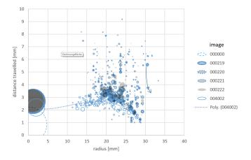
Fig. 11. Travelled distance between  $22^{nd}$  and  $28^{th}ms$  of detachment (000219 to 000222, grey of various outline) against radius from filter center, plus initial (000000 of dashed outline) and final stage (004002 of solid outline). Circle size indicates patch area. Final surface (dotted trendline); at final stage all shown patches are deposited on filter.
