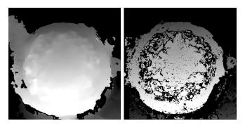
Fig. 2. Disparity map comparison of a machine-learning based stereo matching algorithm [9] (left) and a modified SGM algorithm (right).
