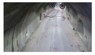
Fig. 1. Subsurface environment at ZaB with ground control points shown in red color for extrinsic camera calibration.
