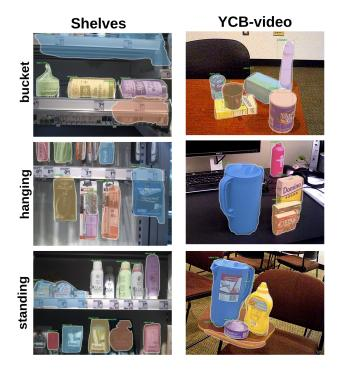
Fig. 2. Class-agnostic instance segmentation results on images of our training set for shelves (left column) and on unseen images of YCB-video [14] (right column).
