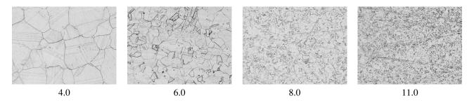
Fig. 2. Samples of varying grain densities. The grain density increases from left to right and exhibits fractal like self similarity at different scales. It does however produce a variety of artifacts due to the etching process depending on size of individual grains and variation among samples. While the grain density is fundamentally a continuum, it is often discretized to whole- or half-grades in practice.
