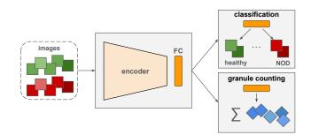
Fig. 2. Proposed architecture to learn classification and/or granule counting.
