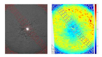
Fig. 6. Depth of particulate layer after filtration, in auto-scaled mm (right). Annotations for top of metal ring and radial profile (red outlines). See the fluctuations beside a radial distribution.
