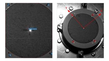
Fig. 3. Crosshair (left) and arrows (right) define origin and orientation of used camera pose-independent right-handed reference coordinate system. For calibration purposes, 11 dedicated reference points with known world coordinates on the filter fixing ring were defined (right). Red circles (right) respectively blue dots (left) mark the selected reference point subset during calibration routine – in particular case marker 1, 6, 8 and 10.
