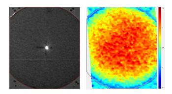
Fig. 5. Left: Image of a fresh, particle-free, flat clamped filter. The reference filter area is outlined red. Black dots represent reference markers. Right: Corrected auto-scaled depth map of the fresh filter area in *mm*. As can be seen, the filter bulges out.
